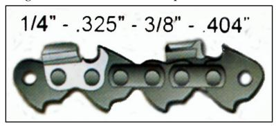
Chain manufacturers identify their chains by pitch, gauge and length. Pitch defines the size of the chain, and determines the thickness of the stone used for sharpening. As when sharpening a chain by hand you must match the file radius to the chain, it also is necessary that the thickness of the grinding stone on the sharpener suits the chain you want to sharpen.
