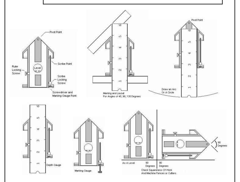
**Special Note:** Sometimes the screwdriver on the scribe does not fit the slot of the pivot screw. This can easily be corrected with a small file by removing any burrs left on the tip from the machining process. Simply filing the flats of the tip a few times will correct the problem.
