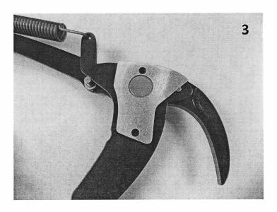
Place spacer as shown in figure 3 and line up screw holes. Place saw blade on spacer *make sure* blade curves away from pulleys as shown in figure 4.
