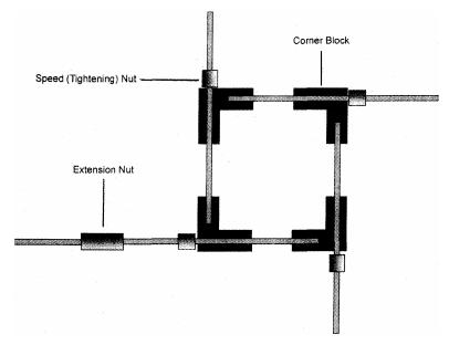
slid along the threaded rod into position at the corner block, where the nut rights itself and the threads engage. The frame is securely held square and true for gluing when the four nuts are tightened against the corner blocks in this manner.
